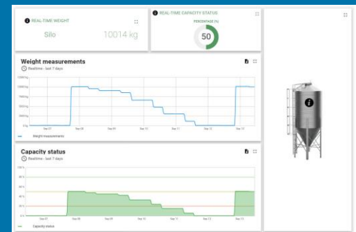
Example of a dashboard with the real time representation of the measured values
